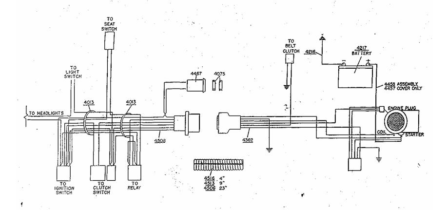
BODY WIRING LOOM - 4508 REAR WIRING LOOM - 4362 WIRING KIT - 8687 (SEE ASSEMBLY BREAKOOWN)
